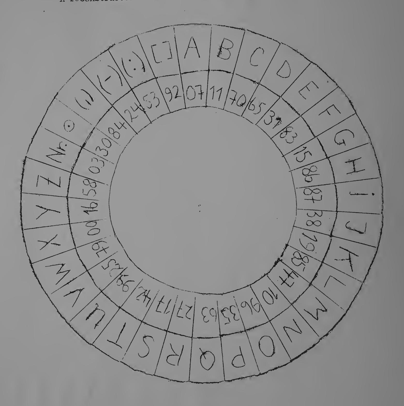
The smaller (red) disc with the reciphering figures was mounted so as to be movable; thus a series of drum (TROMEL) variations could be set.
